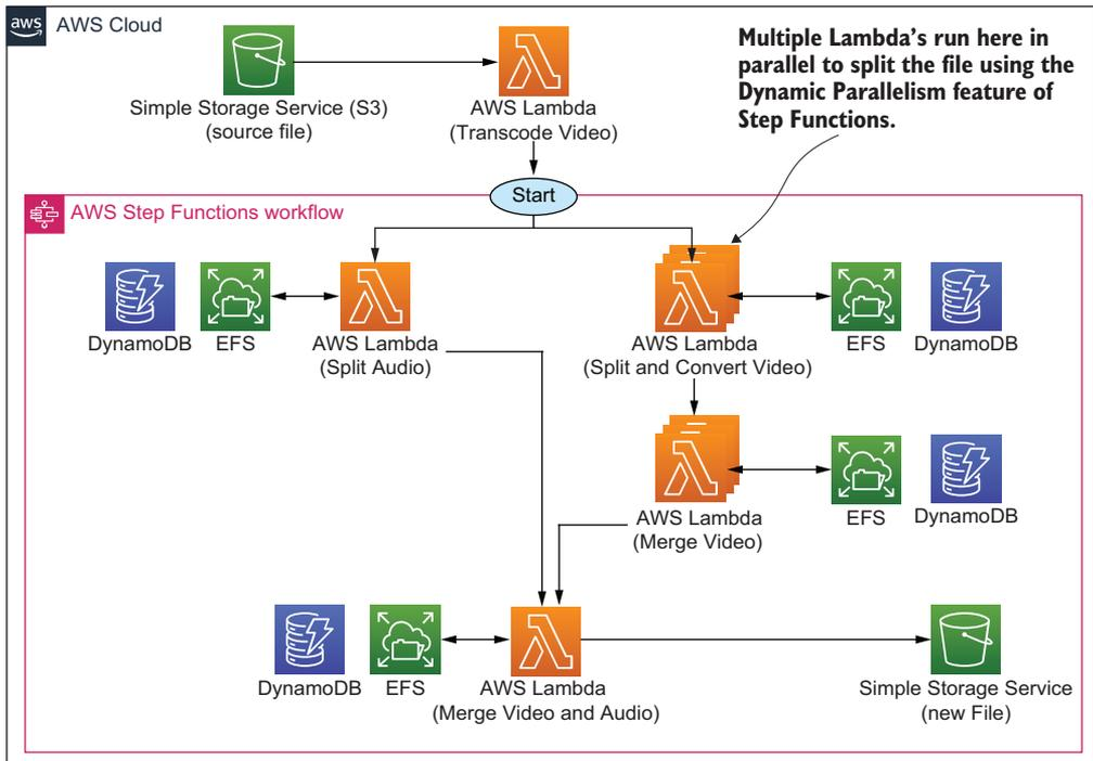
**Figure 8.2** This is a simplified view of the serverless transcoder. There are a few more components to it, but we've avoided including them in this figure to focus on the essential elements of the architecture.
