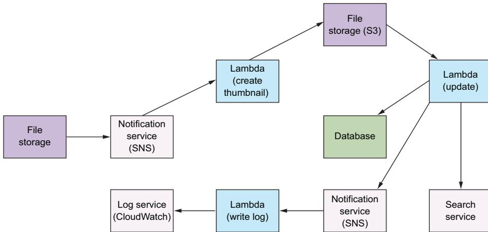
Figure 3.10 The compute-as-gluce architecture uses Lambda functions to connect different services and APIs to achieve a task. In this pipeline, a simple image transformation results in a new file, an update to a database, an update to a search service, and a new entry to a log service.
