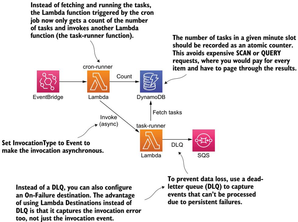
Figure 7.6 An alternative architecture as a solution to our cron job. The solution fans out the processing logic to another function.
