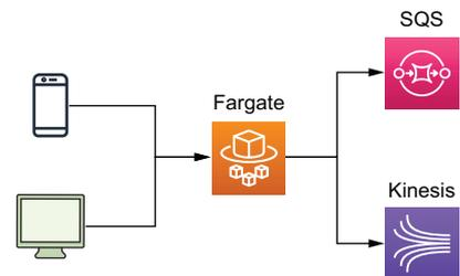
**Figure 6.1** High-level architecture of Yle's ingestion API, which assimilates more than 500 million events per day at a peak throughput of more than 600,000 events per minute. The events are forwarded to Kinesis Data Stream in batches of 500 records. If the Kinesis data stream is unavailable, the events are sent to an SQS dead-letter queue (DLQ) to be reprocessed later.
