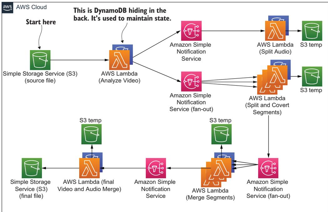
Figure 8.6 The SNS and S3 architecture for the serverless transcoder
