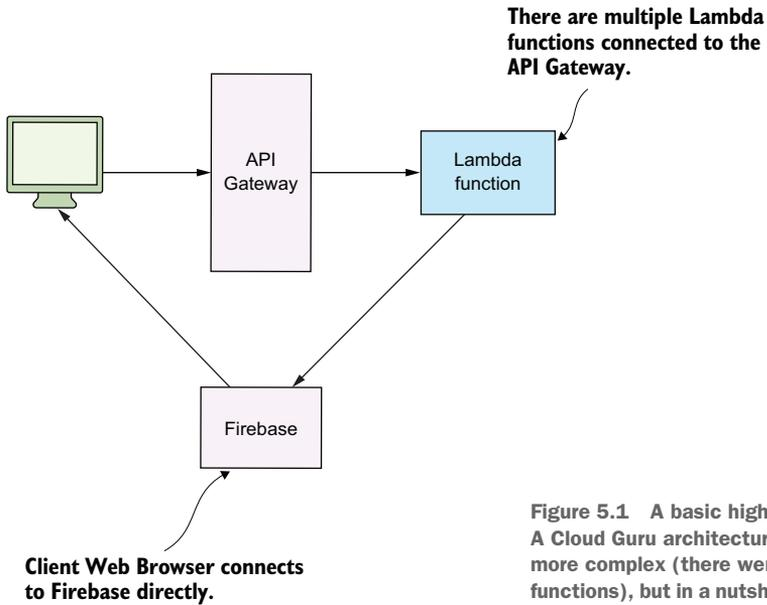
Figure 5.1 A basic high-level view of the initial A Cloud Guru architecture. Their system was more complex (there were many more Lambda functions), but in a nutshell, this is how it worked.
