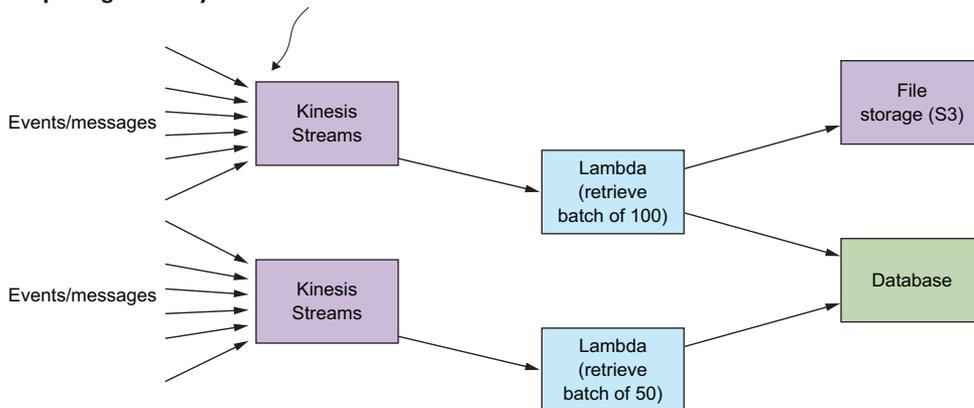
Figure 3.1 Lambda is a perfect tool to process data in near real time.
