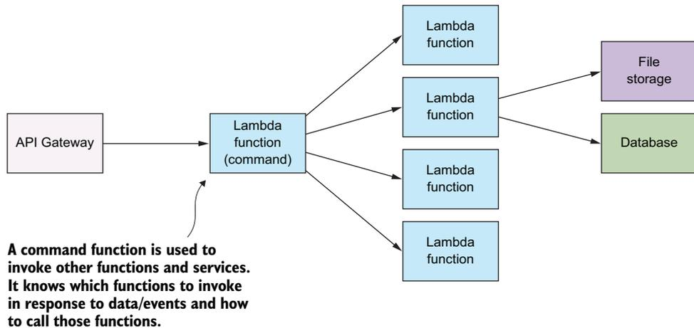
Figure 3.5 The command pattern invokes and controls functions and services from a single function.
