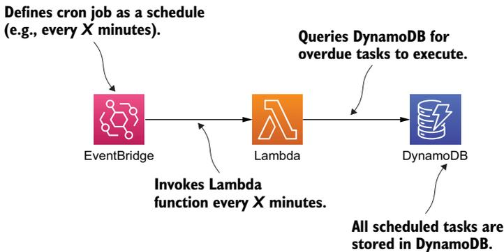
Figure 7.1 High-level architecture showing an EventBridge cron job with Lambda to run ad hoc scheduled tasks.
