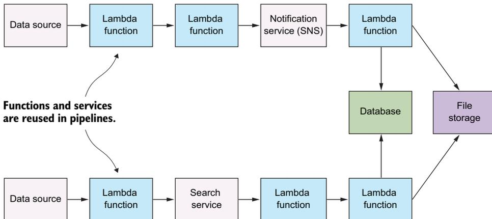
Figure 3.11 The pipes and filters pattern encourages the construction of pipelines to pass and transform data from its origin (pump) to its destination (sink).
