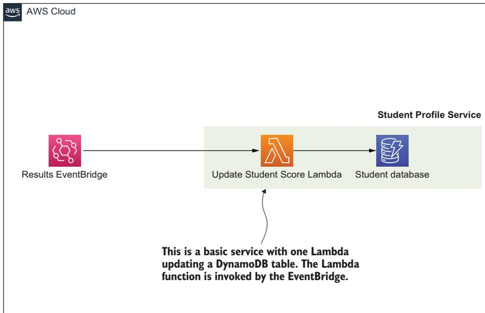
**Figure 9.3** The Student Profile Service is the simplest one in this entire architecture. It's a Lambda function that writes to a Dynamo table.
