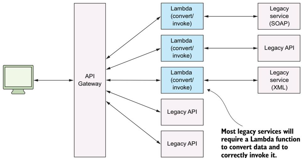
Figure 3.2 We can use the API proxy architecture to build a modern API interface over old services and APIs.
