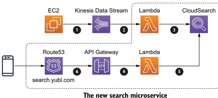
Figure 4.2 A high-level overview of the new architecture running on serverless components
