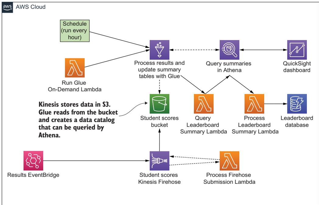
Figure 9.4 The Analytics Service architecture includes Glue, Athena, DynamoDB, Kinesis Firehose, QuickSight, and Lambda.
