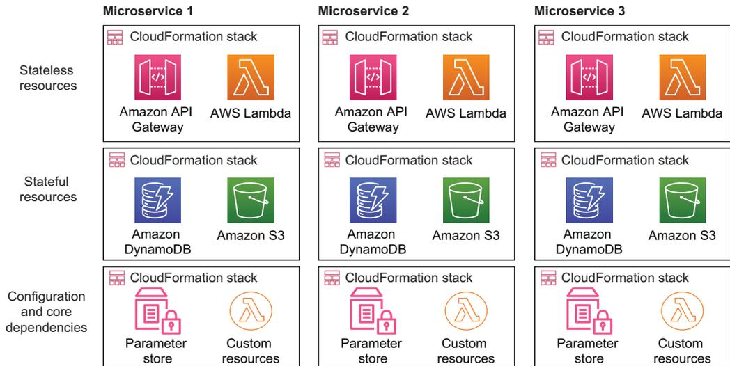
**Figure 5.4** Each microservice is in its own CloudFormation stack, which makes it easy to deploy.
