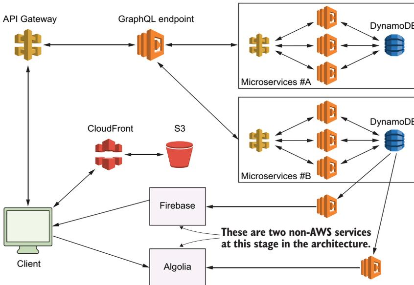
Figure 5.10 A high-level overview of the A Cloud Guru architecture as it was going through a transition
