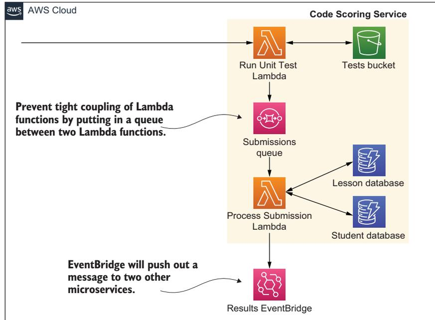
**Figure 9.2** The Code Scoring Service runs the user's code and, if it's successful, kicks off the rest of the chain of events in our system.
