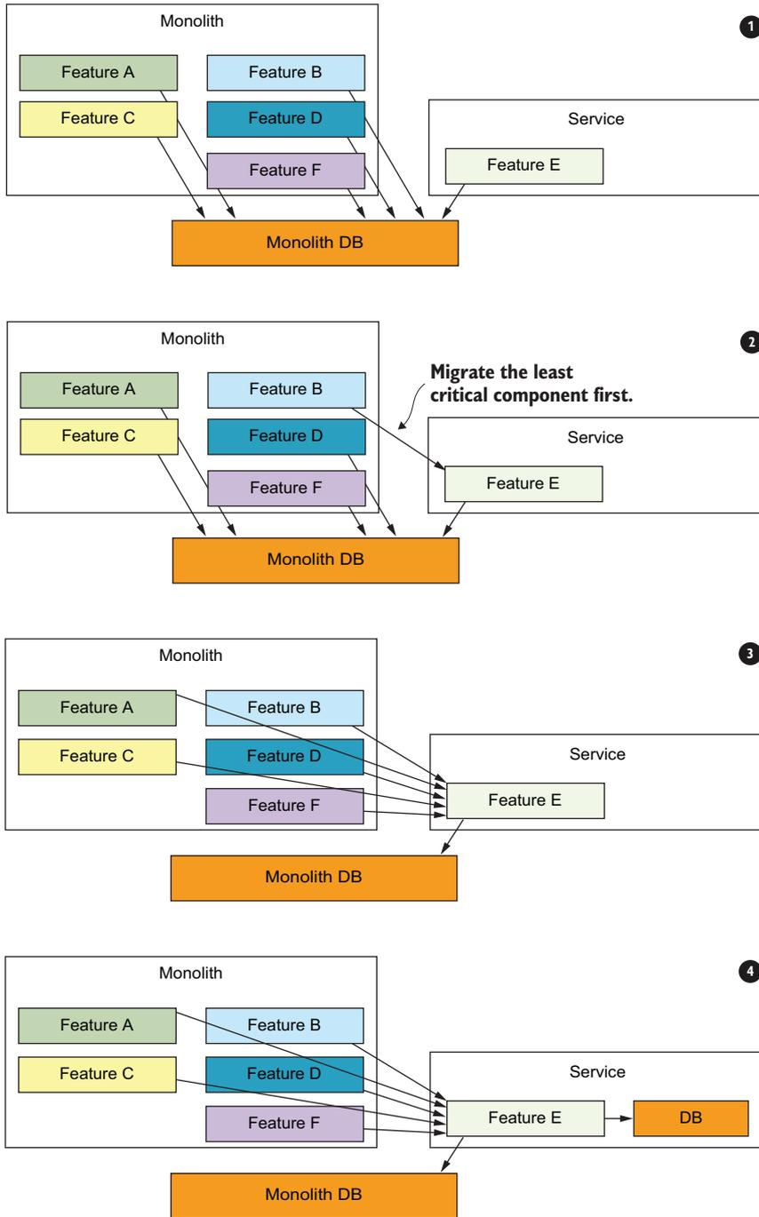
Figure 4.5 Gradually cut off the direct access to the shared monolith database by moving access to go through the new microservice's API instead.
