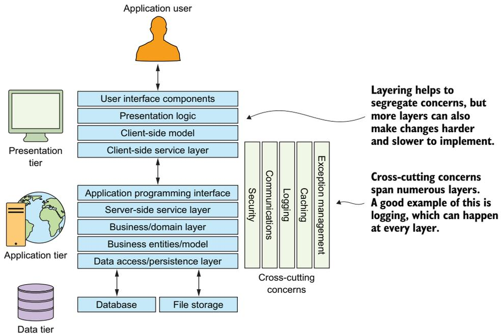
**Figure 1.2** A typical three-tier application is usually made up of presentation, application, and data tiers. A tier can have multiple layers with specific responsibilities.
