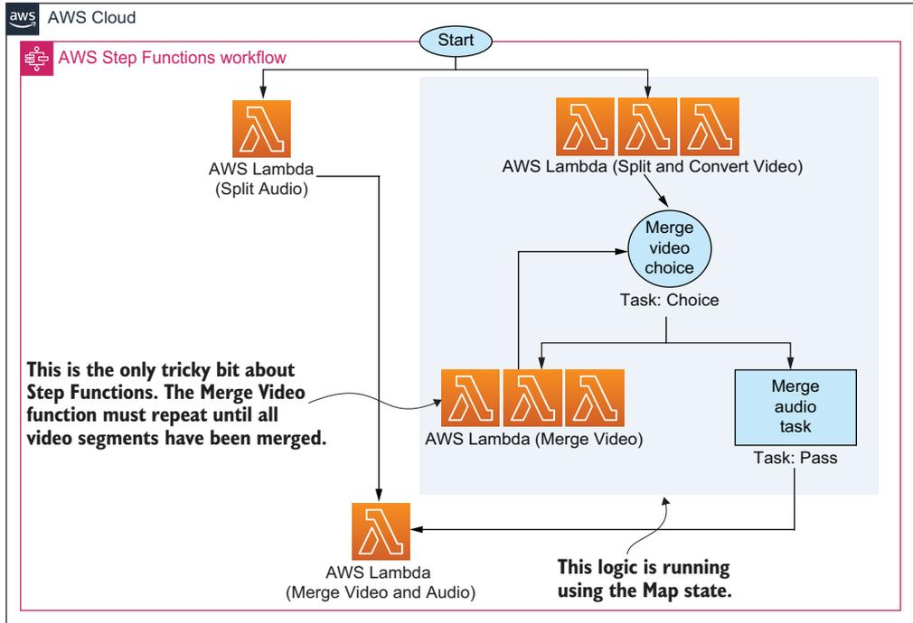
**Figure 8.5** The Step Functions execution workflow does all the work in our transcoder. The video is split, converted, and merged again using two main functions and a bit of logic.
