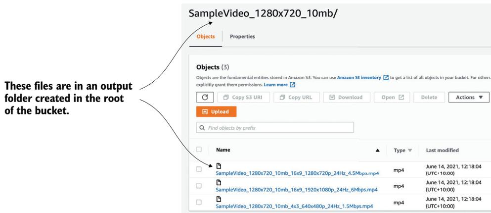
**Figure 2.10** MediaConvert generates three new files and places them in a folder in the transcoded video S3 bucket.
