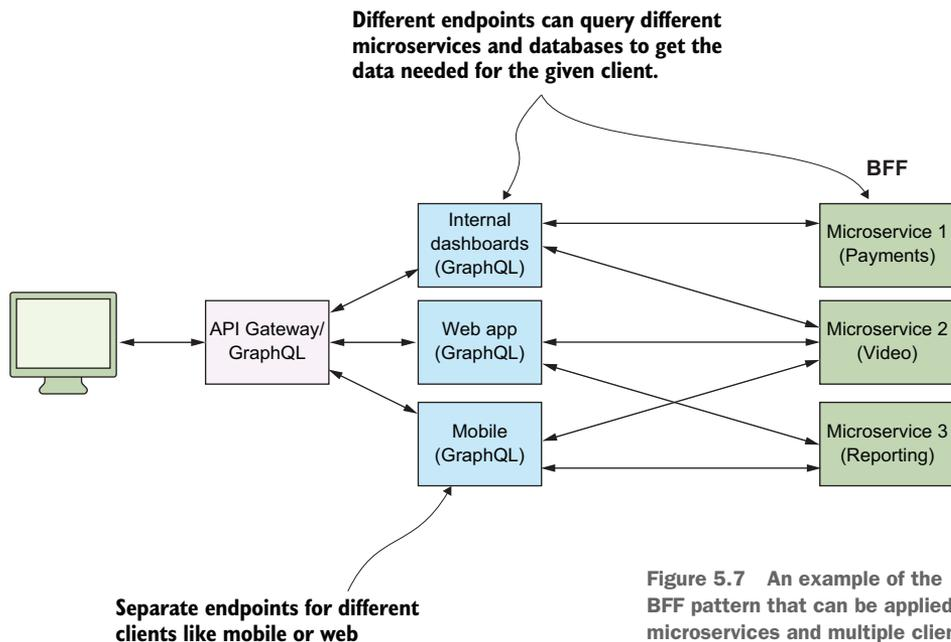
**Figure 5.7** An example of the BFF pattern that can be applied to microservices and multiple clients
