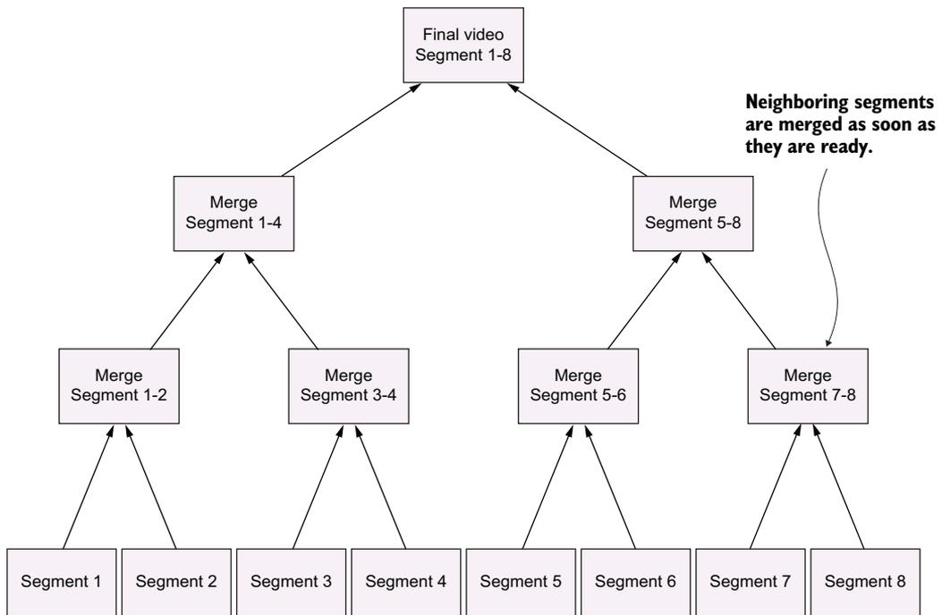
**Figure 8.3** Segments are merged together into a new video. The beauty of our engine is that neighboring segments can be merged as soon as they are ready. There's no need to wait for other, nonrelated, segments to finish processing.
