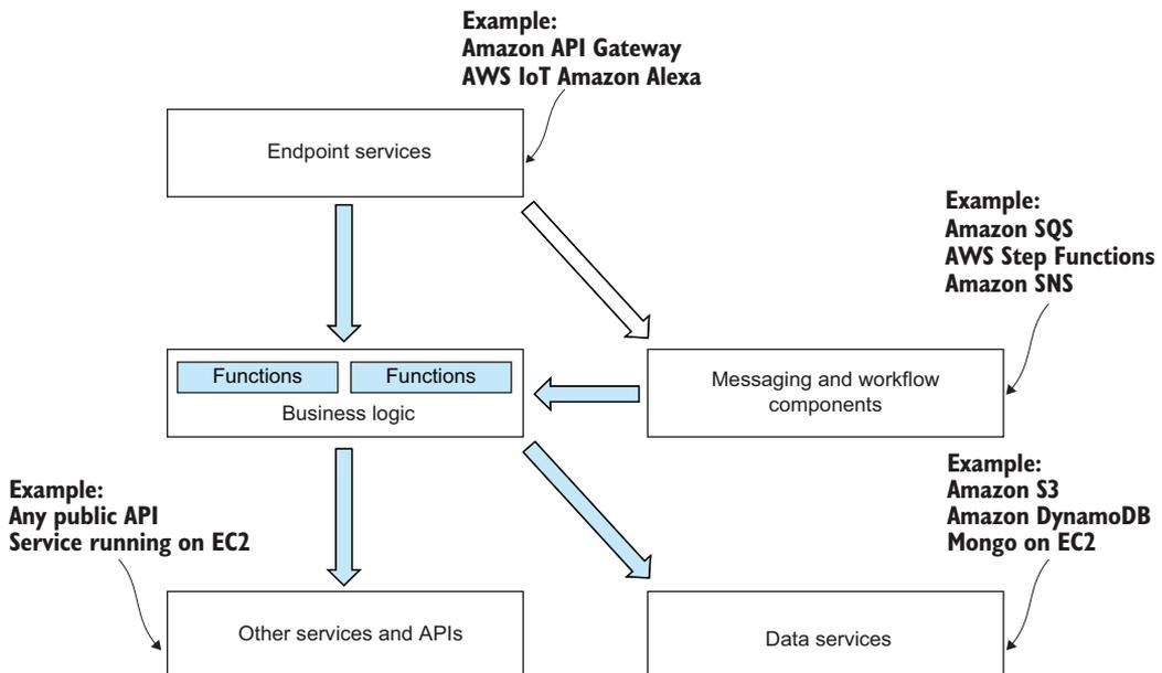
**Figure 10.1** Conceptual architecture of a serverless application
