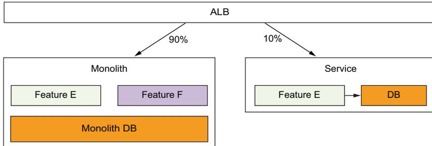
**Figure 4.7** You can use the Application Load Balancer (ALB) to distribute traffic between the monolith and the new microservices. This allows you to minimize impact of unforeseen problems to a subset of users.
