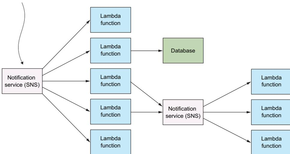
**Figure 3.9** The fan-out pattern is useful because many AWS services (such as S3) can't invoke more than one Lambda function at a time when an event takes place.
