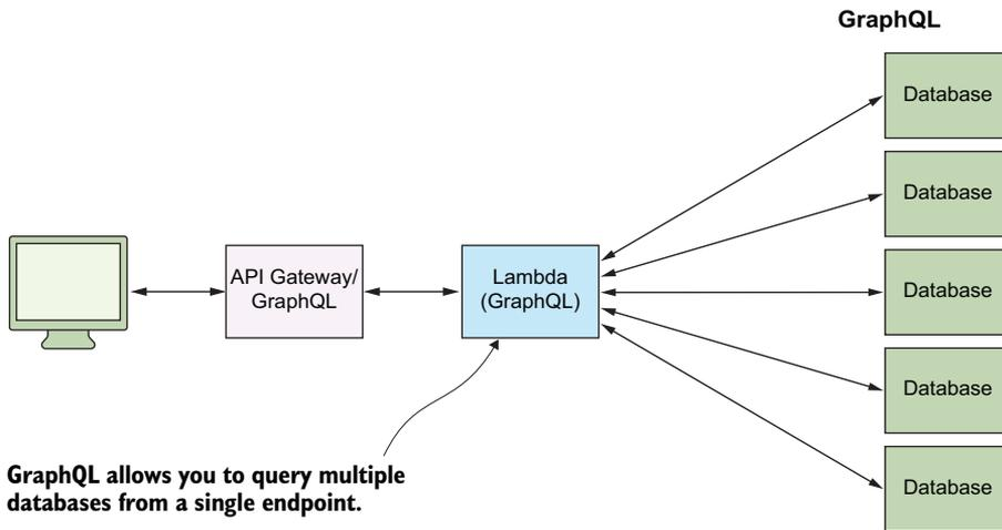
**Figure 5.6** A GraphQL library running in a Lambda function can query multiple databases and, using schema stitching, produce a result relevant for each individual client.
