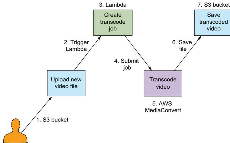
**Figure 2.1** The *24-Hour Video* backend is built with AWS S3, MediaConvert, and Lambda. This pipeline may seem to have a lot of steps initially, but in this chapter, we'll break this down, and you'll build a scalable serverless system in no time at all.
