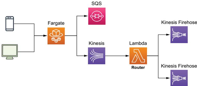
**Figure 6.2** The Lambda Router function routes events to different Kinesis Firehose streams so they can be aggregated and converted to Apache Parquet files.
