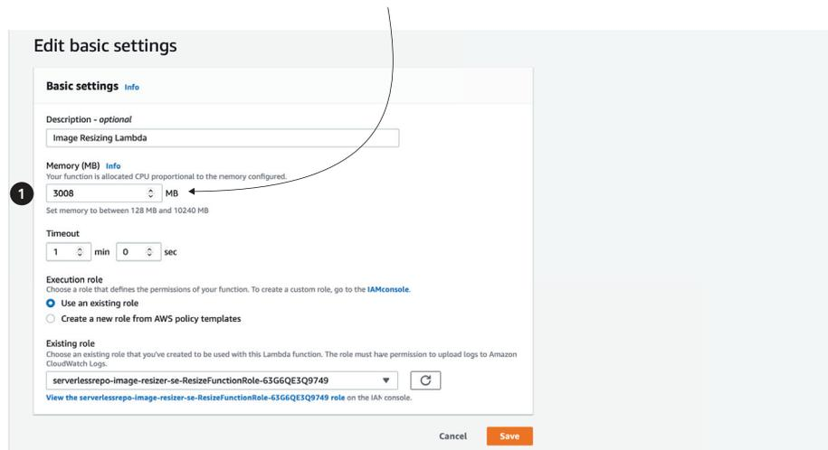
**Figure 10.10** In Edit Basic Settings, you can adjust the amount of memory allocated to the function.
