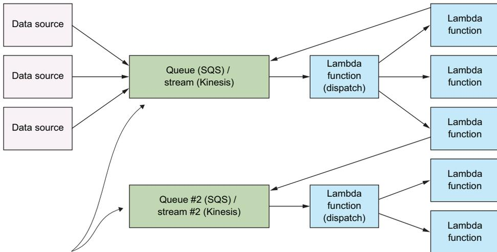
**Use multiple queues/streams to decouple multiple components in your system.**
