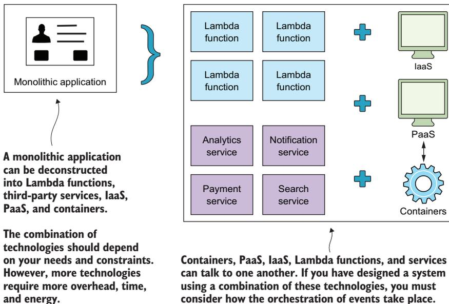
**Figure 1.3** Serverless architecture is not an all-or-nothing proposition. If you currently have a monolithic application, you can begin to gradually extract components and run them in isolated services or compute functions. You can decouple a monolithic application into an assortment of IaaS, PaaS, containers, functions, and third-party services if it helps.
