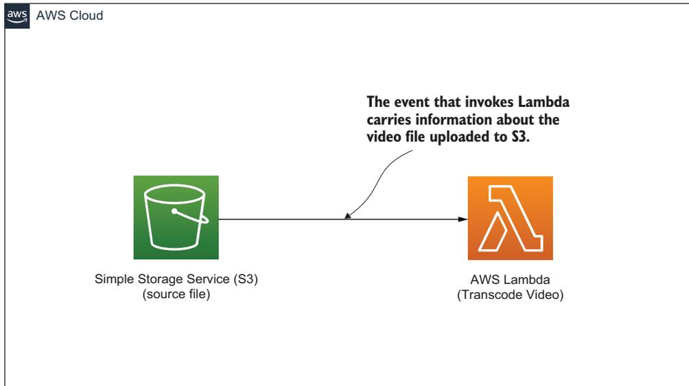
**Figure 8.4** This is a basic and common serverless architecture. Invoking code from S3 is the bread and butter of Lambda functions.
