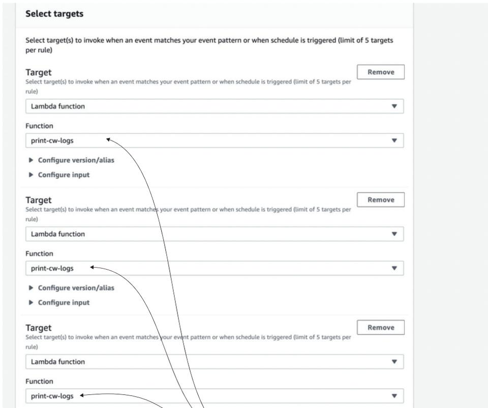
The same function can be configured as a target more than once. Each time the cron job runs, the function would be invoked multiple times, one for every time it's configured as a target.
