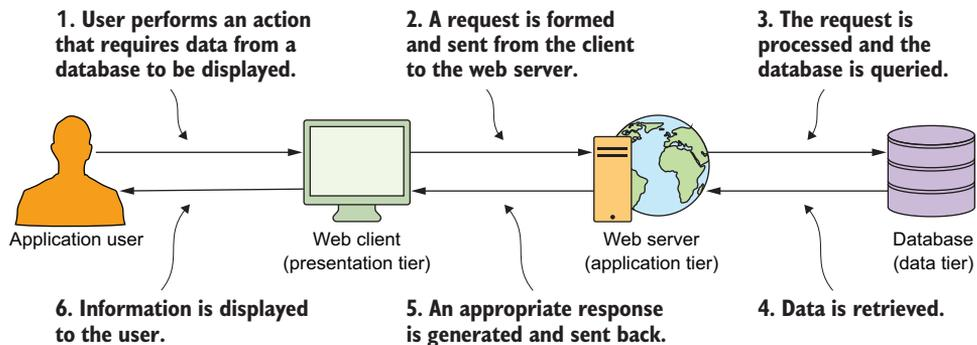
**Figure 1.1** A basic request-response (client-server) message-exchange pattern that most developers are familiar with. There’s only one web server and one database in this figure. Most systems are much more complex.
